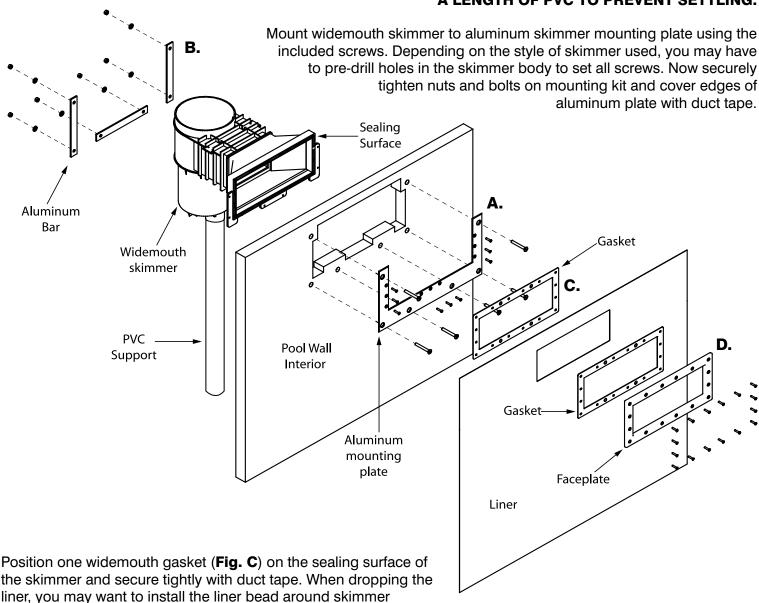
After liner has been installed and water level approaches skimmer, prep skimmer faceplate (**Fig. D**) by lining up faceplate and gasket, and then carefully drive screws through faceplate, gasket, liner, interior gasket and into skimmer throat. Securing the corners first will help ensure correct placement.
